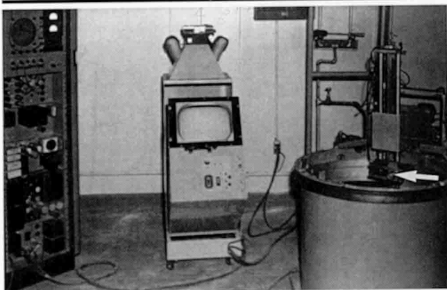
Figure 1. Photograph of Dr Howry's early water bath scanner (1953–1954), with the transducer (arrow) mounted on a ring within the water bath scanner so that it could be moved 360° around the patient. The electronic system is on the left and the display oscilloscope is in the center.
